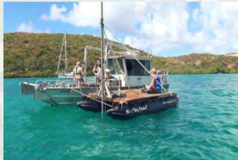
EM61 Deep Floating Platform
