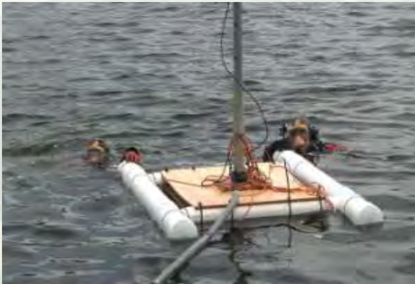
EM61 Deep and Shallow Floating Platforms
