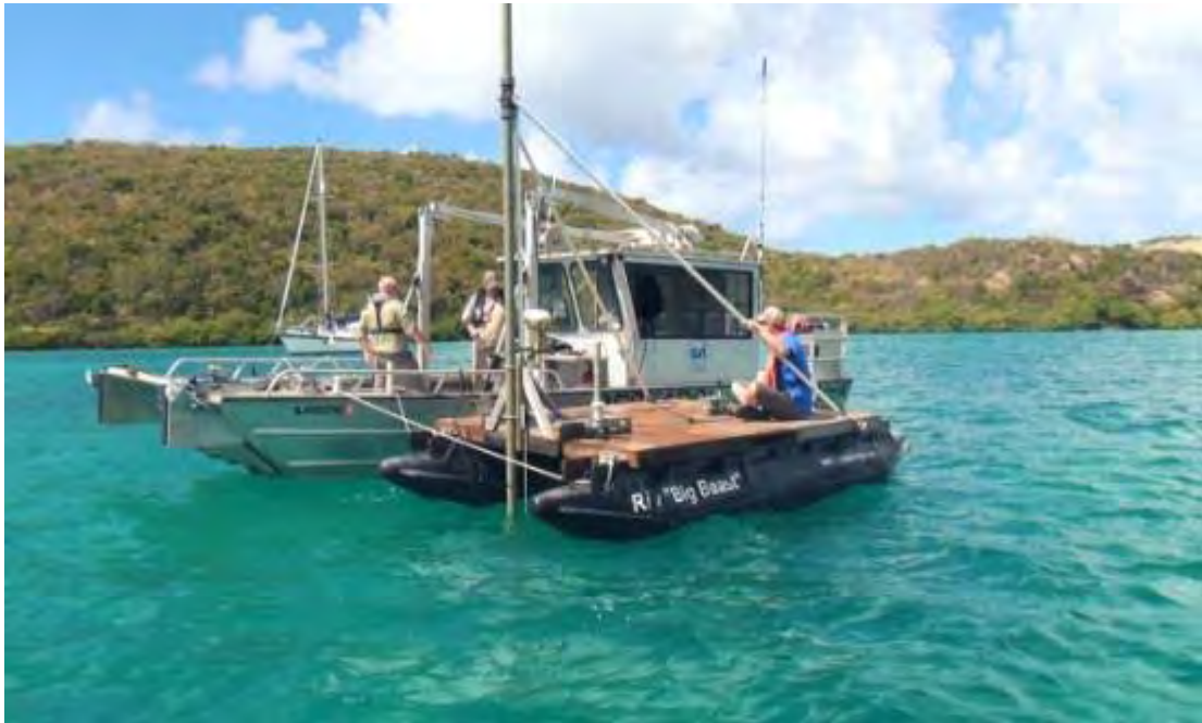
Figure 3-2: EM61 Deep Floating Platform
