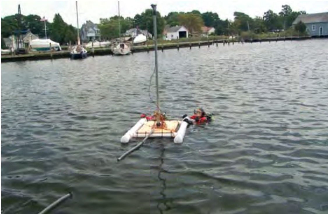
Figure 3-1: EM61 Deep and Shallow Floating Platforms
